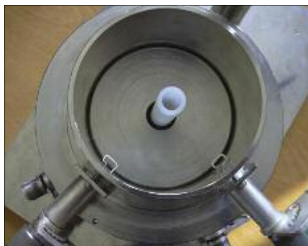
Figure 2: Cavity resonator and sample holder
