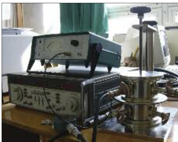
Figure 1: A measuring system utilizing a cavity resonator
