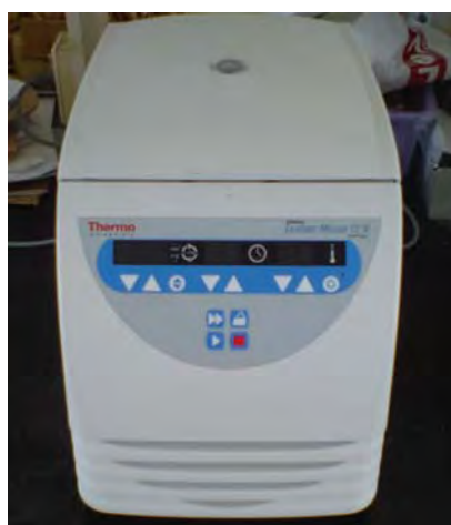
Figure 1. Refrigerated centrifuge apparatus
